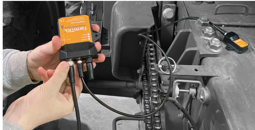
Sensor A connected with CAN wire and CAN terminator
