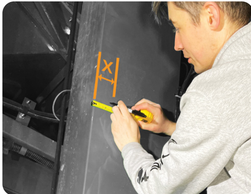
Distance (X) from the back of the clean grain elevator to the center of the drill hole
